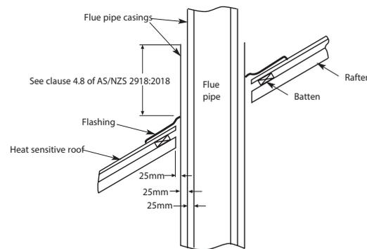
Figure 8 REFERENCE : AS2918:2018 FIGURE 4.8 - EXAMPLE OF ROOF PENETRATION
