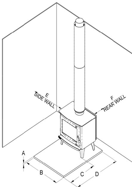
Figure 2 - Corner Installation
